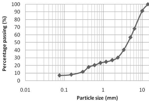
Fig. 1: Particle size distribution curve of laterite.
