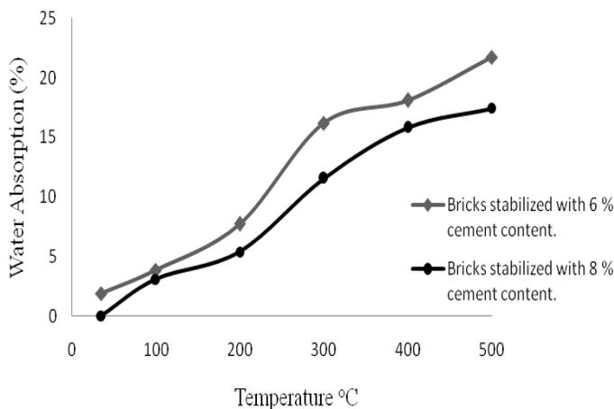
Fig.3: Variation of Water Absorption with Temperature.
