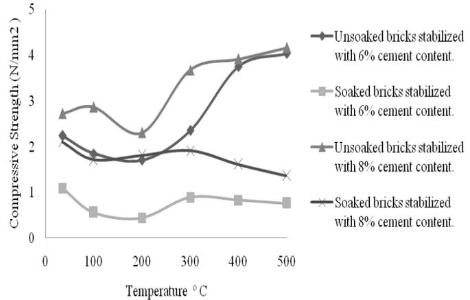
Fig. 2 : Variation of compressive strength with Temperature.
