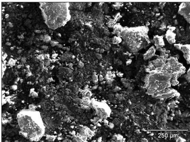
Figure 5: SEM image of the various mineral particles
