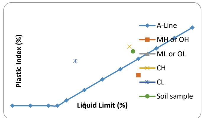
**Figure 6: Plasticity Chart for Soil Classification**
