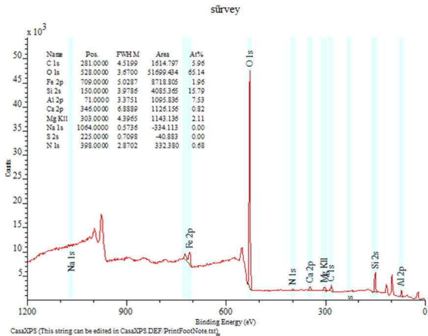
Figure 3: XPS Spectrum of surface elemental composition
