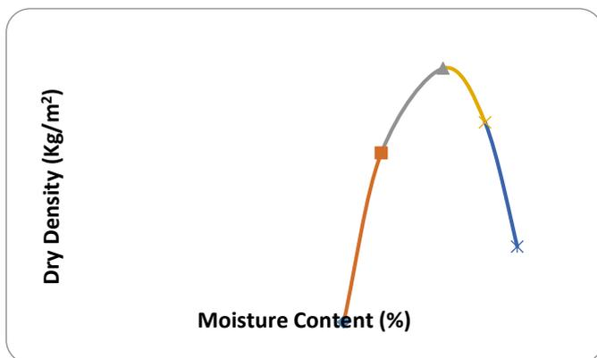
Figure 7: Moisture - dry density relationship for the soil sample
