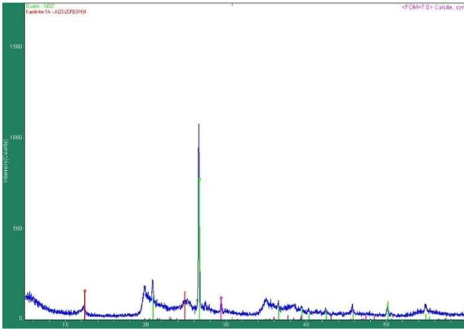
Figure 2: XRD Diffractogram of the soil sample indicating Quartz and Kaolinite
