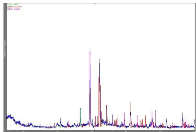
**Figure 1: XRD Diffractogram of the soil sample indicating Quartz, Larnite and Calcite**
