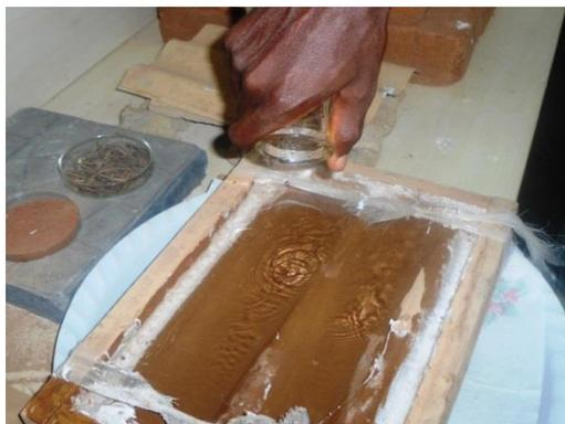
Figure 4: Sample tested for water penetration
