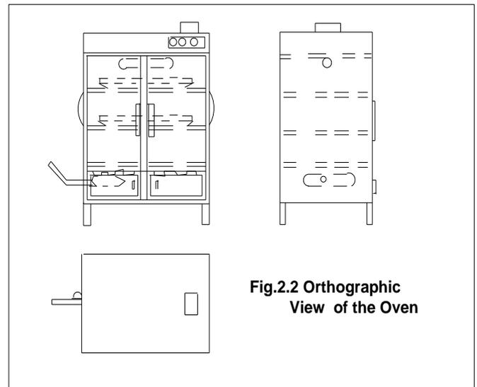
Fig.2.2 Orthographic View of the Oven
