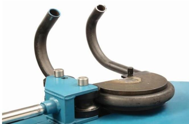
**Fig. 1.0 Pipe Bending Process**
