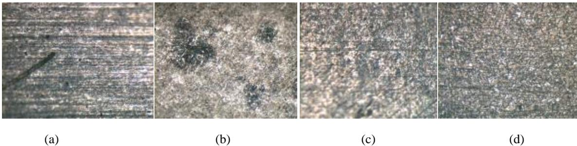
**Plate 2: Micrographs of mild steel austenised at 850°C, quenched in water and tempered at (a) 250°C (b) 350°C (c) 450°C (d) 550°C. The structure developed contain more lower bainite crystals compared to specimens austenised at 800°C.**
