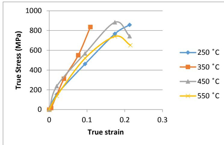
Figure 1d: Effect of tempering temperature on the tensile behaviour of mild steel austenised at 950<sup>0</sup>
