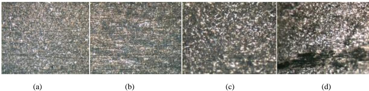
**Plate 4:** Micrographs of mild steel austenised at 950°C, quenched in water and tempered at (a) 250°C (b) 350°C (c) 450°C (d) 550°C. The microstructures consist of lower bainite particles whose size reduces as the tempering temperature increases except at 350°C..
