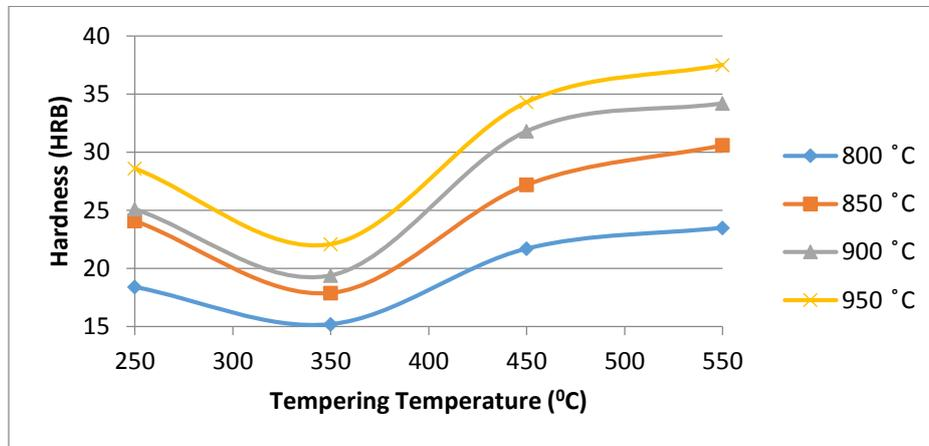
Figure 3: Effect of tempering on the hardness of mild steel austenitised at varying temperatures
