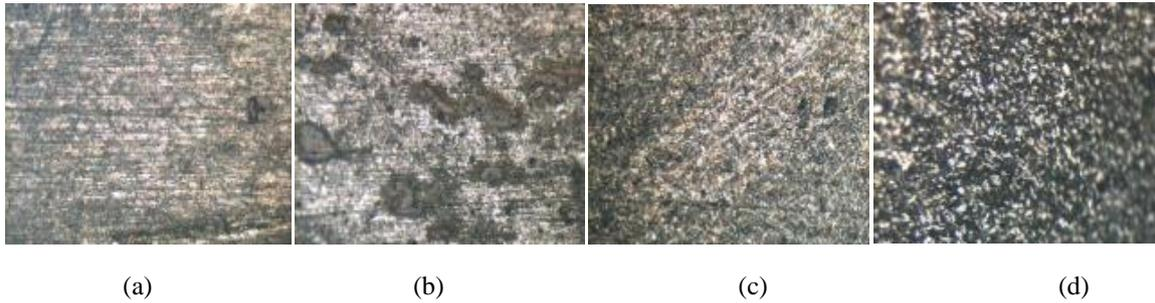
**Plate 3:** Micrographs of mild steel austenised at 900°C, quenched in water and tempered at (a) 250°C (b) 350°C (c) 450°C (d) 550°C. The microstructures consist of lower bainite showing needle-like carbide particles whose size reduces as the tempering temperature increases except at 350°C..
