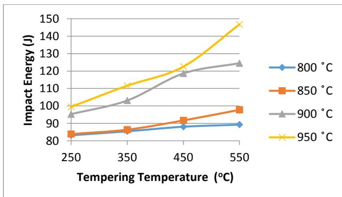
Figure 2: Effect of tempering on the impact energy of mild steel austenised at varying temperatures
