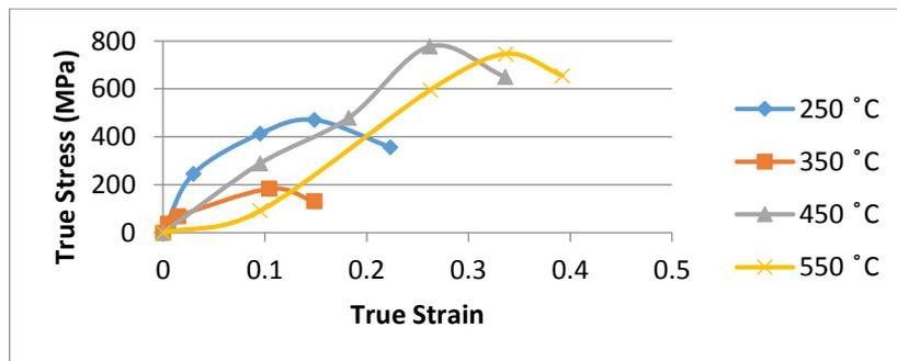
**Figure 1a:** Effect of tempering temperature on the tensile behaviour of mild steel austenised at 800°C
