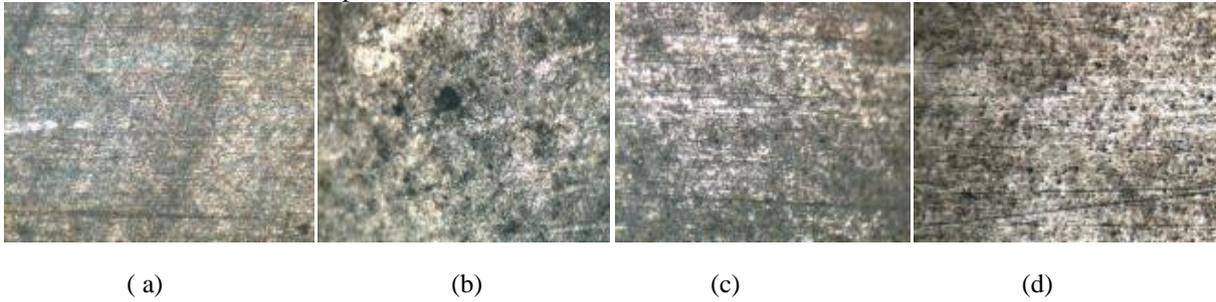
**Plate 1: Micrographs of mild steel austenised at 800°C, quenched in water and tempered at (a) 250°C (b) 350°C (c) 450°C (d) 550°C. The microstructures consist of fringes of lower bainite but a preponderance of pearlite showing progressive reduction in size as the tempering temperature increases.**
