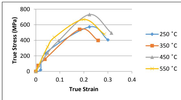
**Figure 1b: Effect of tempering temperature on the tensile behaviour of mild steel austenised at 850<sup>o</sup>C**
