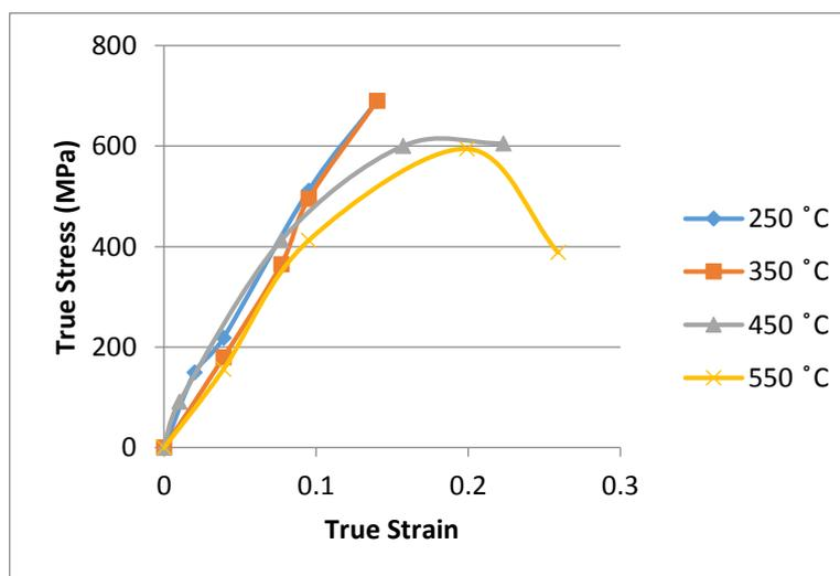
**Figure 1c: Effect of tempering temperature on Effect of tempering temperature on the tensile behaviour of mild steel austenised at 900<sup>o</sup>C**
