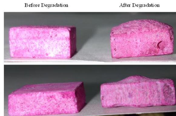
Fig. 7: Swelling of the blend with 7.5% and 10% chitosan after 35 days of degradation.
