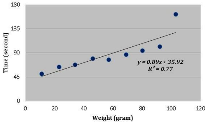
Figure 4: The weight of tire tubes against time for 9 experiment cycles
