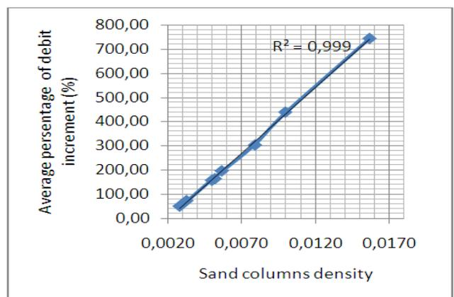
Fig. 7 Relationship of the average percentage of debit increment with the sand columns density
