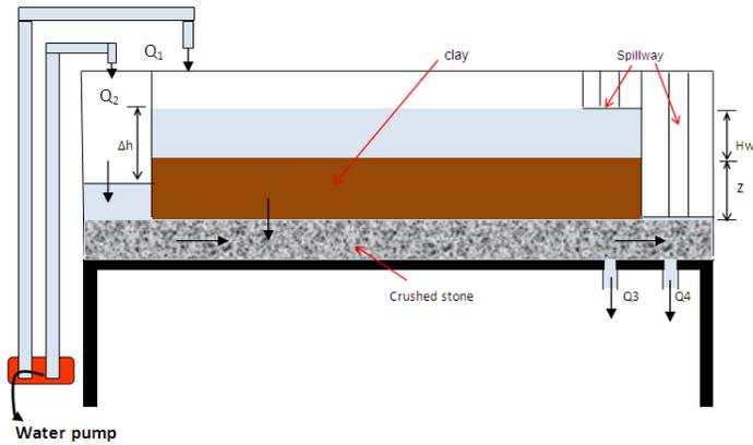
Fig. 2 : Physical recharge reservoir model testing without sand columns
