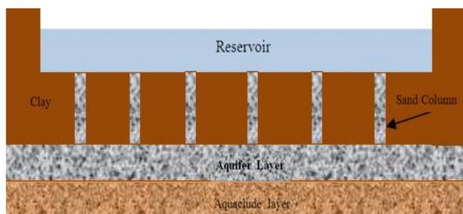
**Fig. 1 The concept of recharge reservoir with sand columns**
