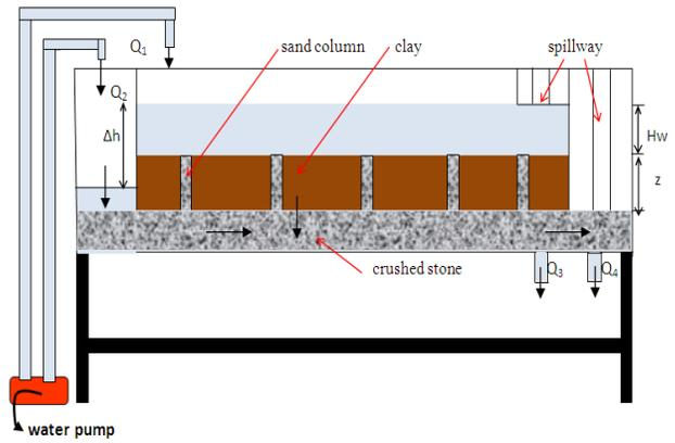
Fig. 3 Physical recharge reservoir model testing with sand columns
