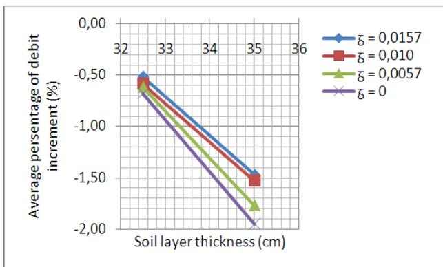
Fig. 5 Relationship of the average percentage of debit increment with the soil layer thickness (z)
