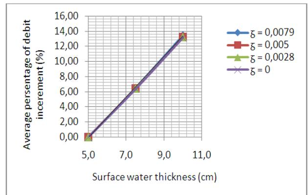
Fig. 6 Relationship of the average percentage of debit increment with the surface water thickness
