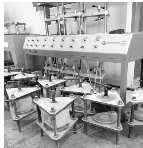
Fig. 2: Water penetration test set up
