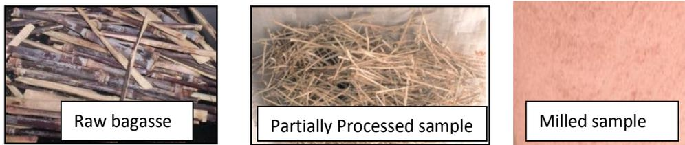
Plate 1: Preparation of sugarcane bagasse for analyses
