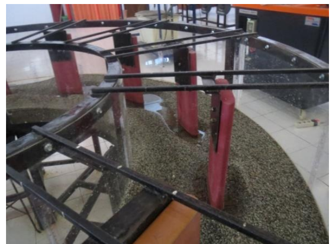
Figure 7: Coordinates installation of pillars at each intervals of 30^{\circ}
