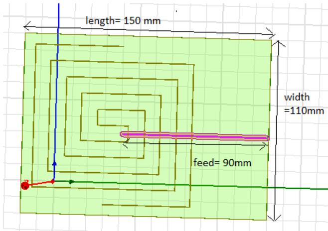
Fig. 2. Feed touching the center of double-arm spiral antenna
