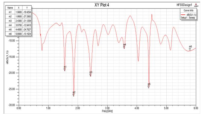
**Fig. 7: Return loss vs frequency of single arm spiral slot antenna.**
