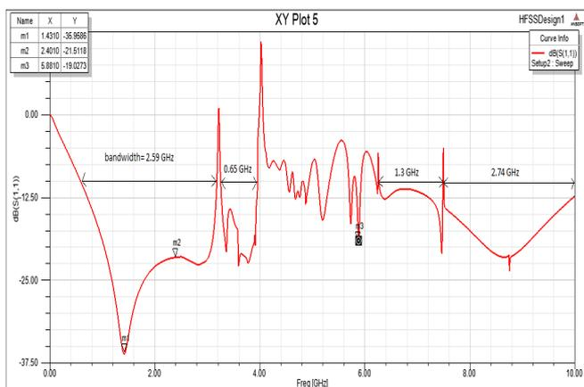
**Fig. 6: Return loss vs frequency of double arm spiral slot antenna.**
