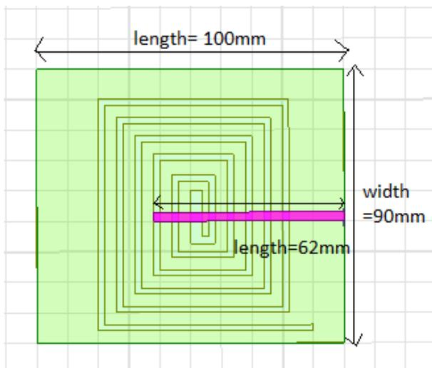
Fig. 4. Single arm spiral antenna with optimized feed length.
