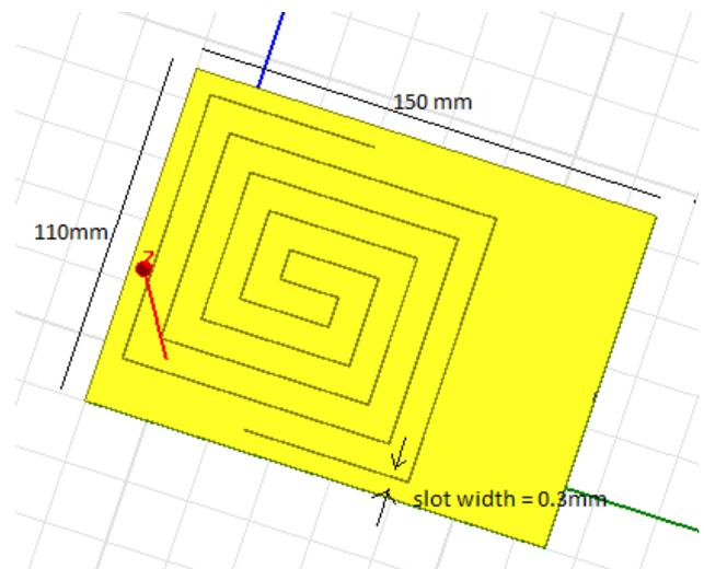
Fig. 1. Top View Of Double Arm Spiral
