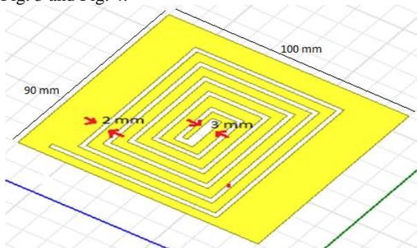
Fig. 3. Top View Of Single Arm Spiral.
