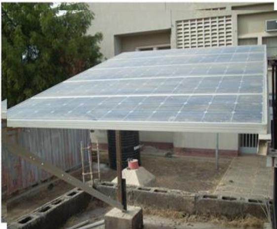
**Fig. 2: experimental photovoltaic array (built from m55 siemens modules)**
