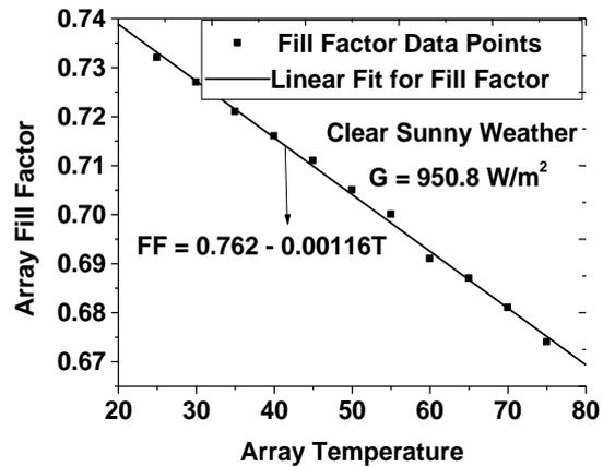
Fig. 10: array fill factor as function of temperature at clear sunny season average irradiance
