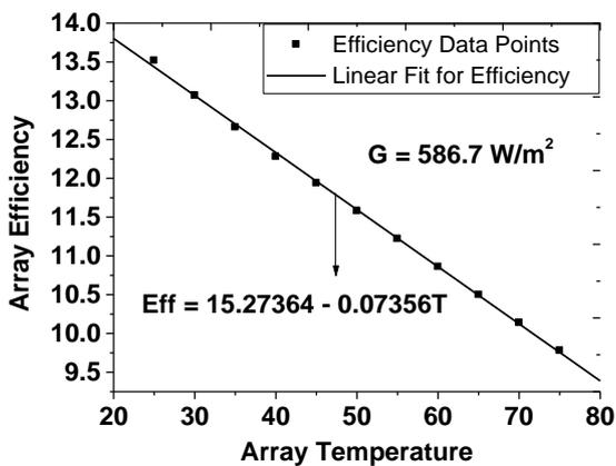
Fig. 4: array energy conversion efficiency as function of temperature at harmattan season average irradiance
