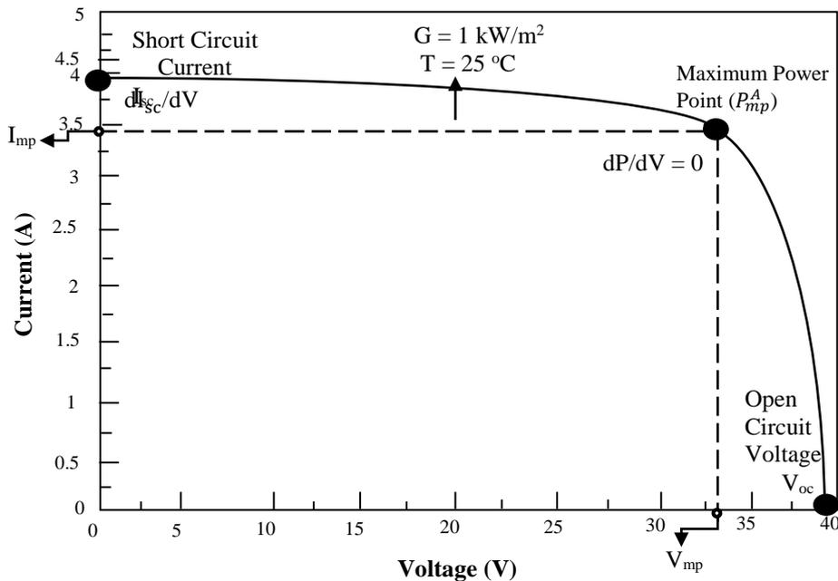
Fig. 1: location of points of interest needed for calculating Energy conversion efficiency and fill factor of an array
