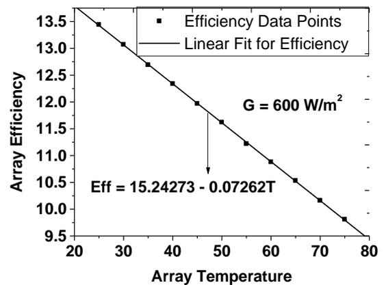
Fig. 5: array energy conversion efficiency as function of temperature at cloudy season average irradiance
