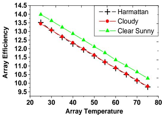
Fig. 7: combined array conversion efficiencies as function of temperature at harmattan, cloudy and clear sunny season average irradiances
