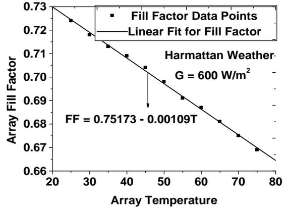
Fig. 9: array fill factor as function of temperature at cloudy season average irradiance
