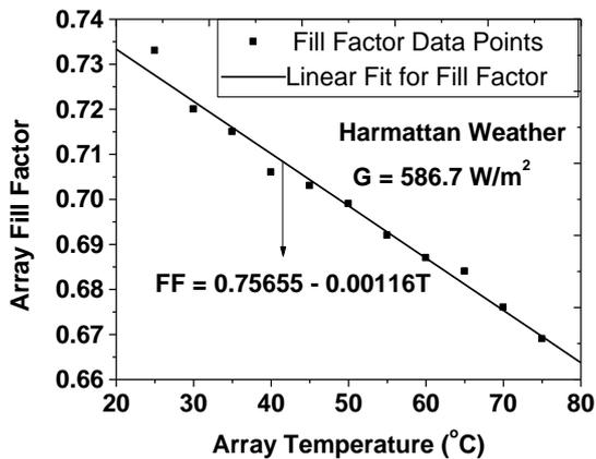
Fig. 8: array fill factor as function of temperature at harmattan season average irradiance
