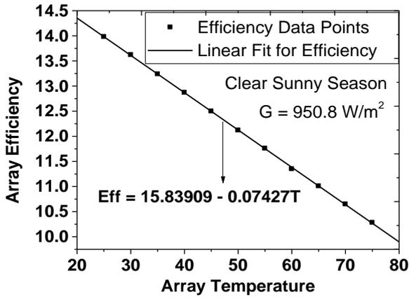
Fig. 6: array energy conversion efficiency as function of temperature at clear sunny season average irradiance
