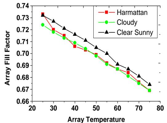
Fig. 11: combined array fill factors as function of temperature at harmattan, cloudy and clear sunny season average irradiances
