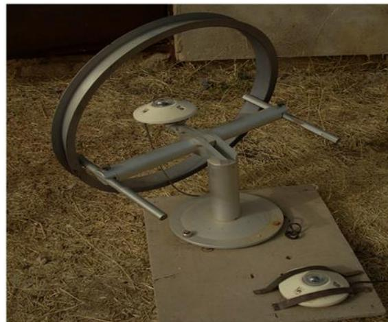
**Fig. 3: pyranometer (model no.: cm6b) for Direct solar radiation measurements**
