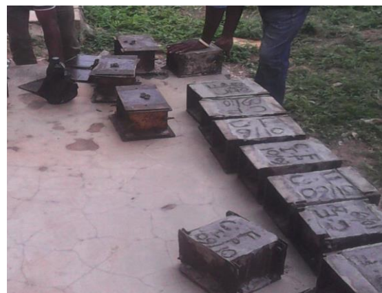
Plate 1d: Preparation of Concrete Cubes from the Different Mix Methods
