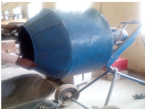
Plate 1c: Concrete Mixing using Mixing Machine
