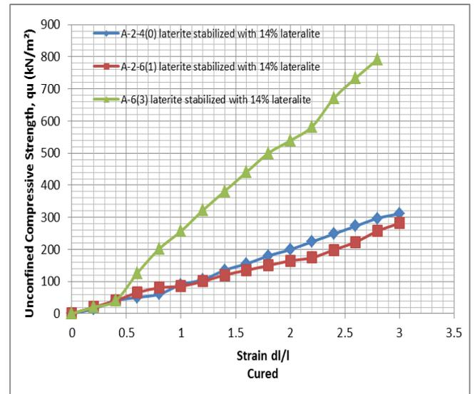
Figure 9: Curves of relationship between UCS and strain for air cured 14% soil-lateralite stabilization
