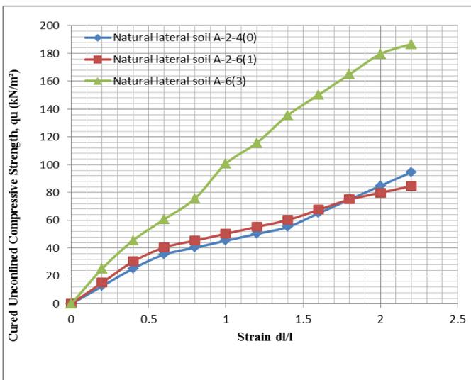
Figure 7: Curves of relationship between UCS and strain of air cured natural laterite soil
