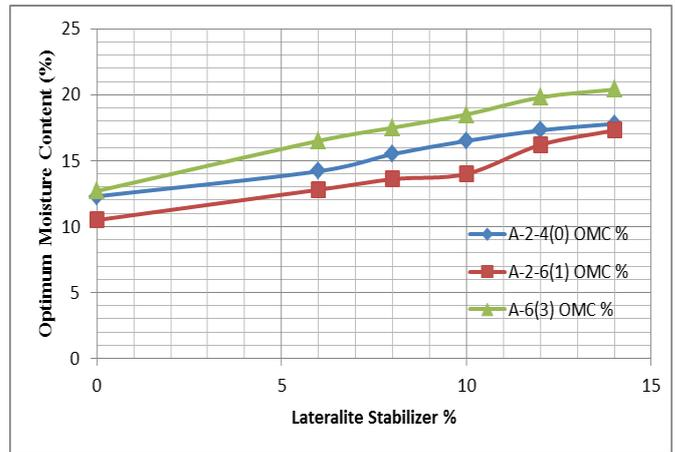
**Figure 2: Curves of relationship between OMC and percent increase of soil-lateralite stabilization**
