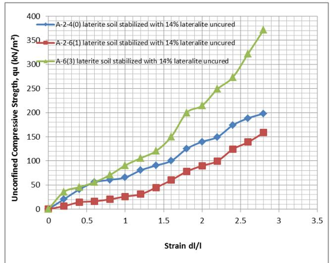
Figure 8: Curves of relationship between UCS and strain for uncured 14% soil-lateralite stabilization
