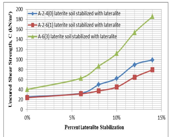
Figure 10: Curves of relationship between shear strength and percent of uncured soil-lateralite stabilization
