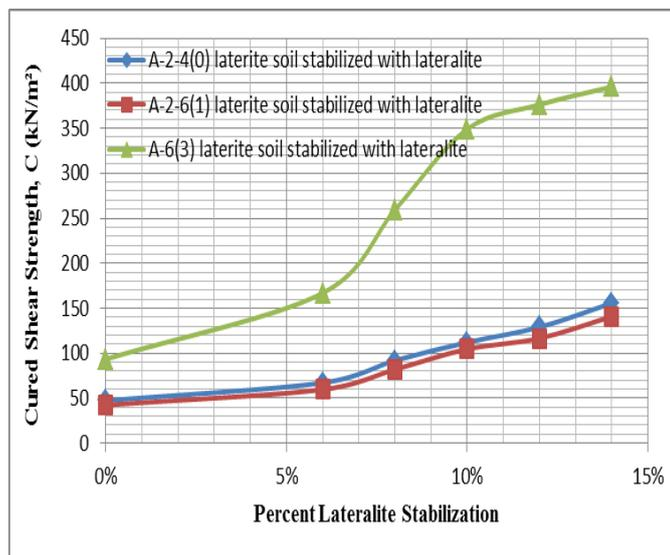
Figure 11: Curves of relationship between shear strength and percent of cured soil-lateralite stabilization
