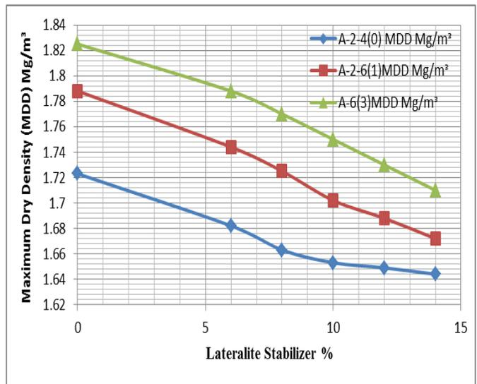
**Figure 3: Curves of relationship between MDD and percent increase of soil-lateralite stabilization**
