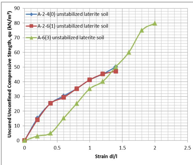
Figure 6: Curves of relationship between UCS and strain of uncured natural laterite soil
