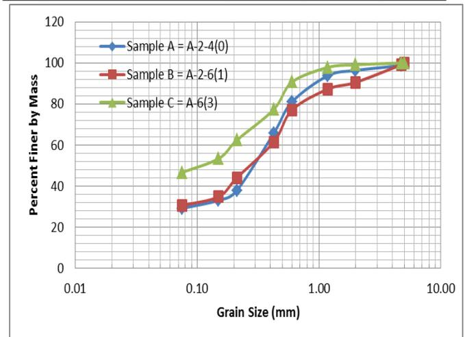
Figure 1: Grain size analysis for the three selected natural laterite soil samples
