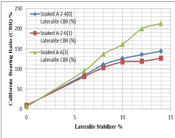
Figure 5: Curves of relationship between CBR and percent increase of soaked stabilized soil-lateralite
