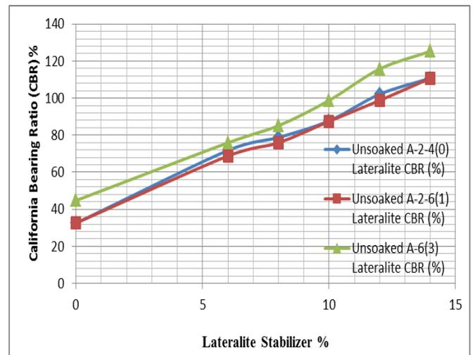
**Figure 4: Curves of relationship between CBR and percent increase of unsoaked stabilized soil-lateralite**
