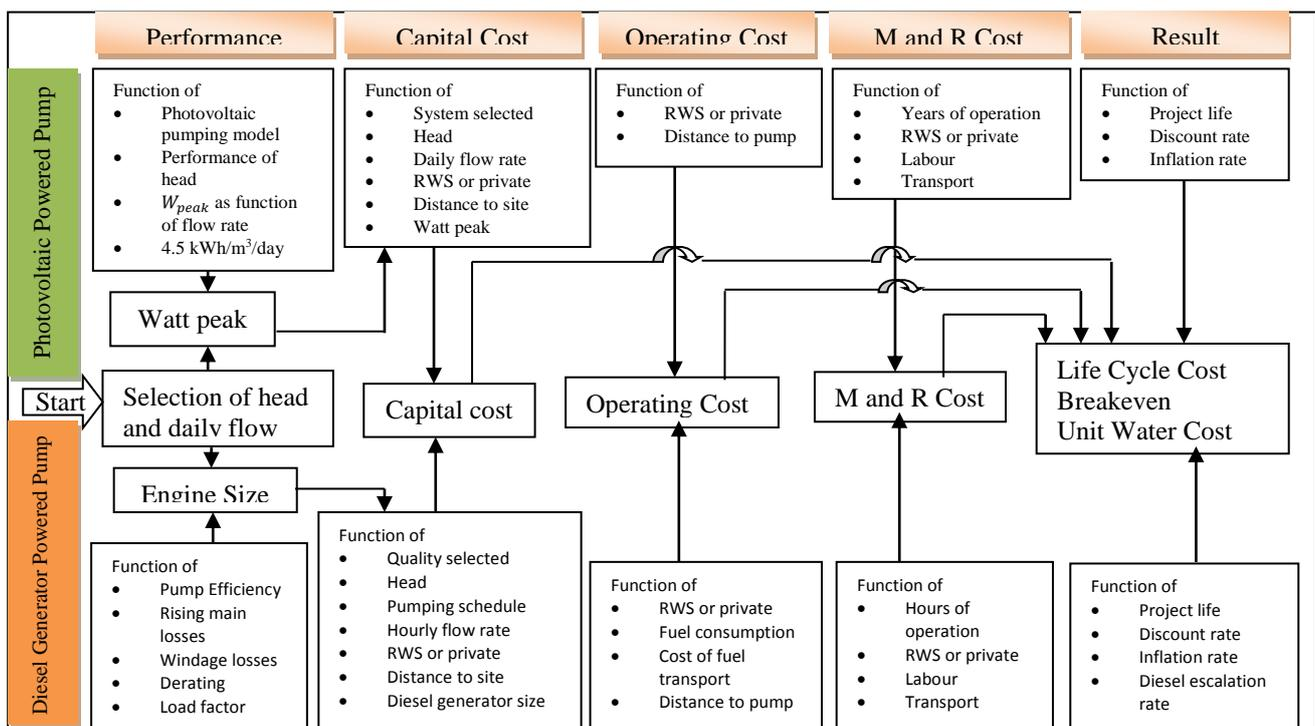
**Figure 3: Spreadsheet Life Cycle Costing**
