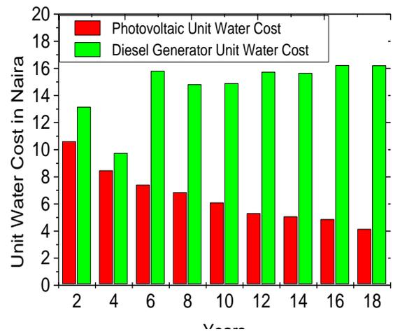
Figure 5: Photovoltaic versus Diesel Generator Powered Pump Life Cycle Cost Comparison.
