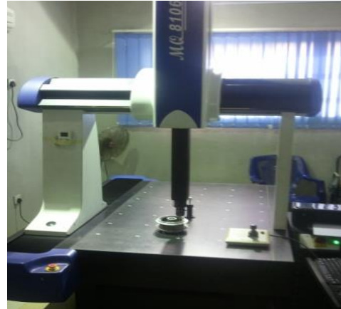
Figure 2.4 Measurement set up on the hub
