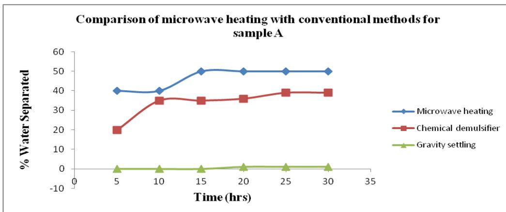
Figure 8a: Comparison of microwave heating with conventional methods.
