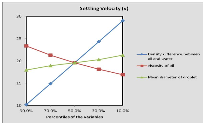
Figure10: Spider chart showing degree of variance of parameters on settling velocity
