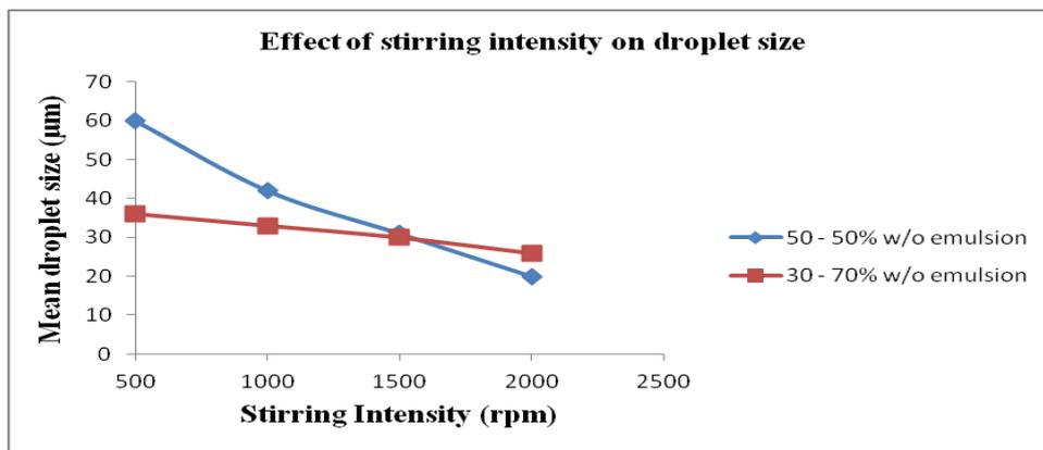
Figure 3: Effect of stirring intensity on droplet size
