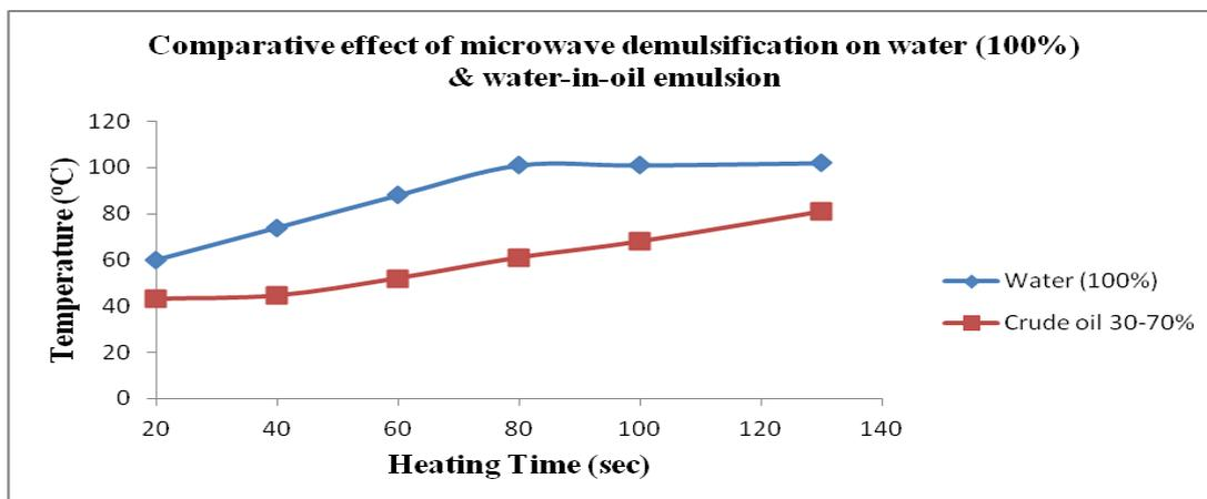
Figure.5: Comparative effect of microwave demulsification on water (100%) & water-in-oil emulsion
