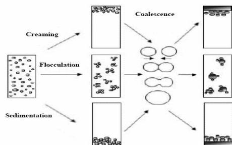
**Figure1: Processes Taking Place in an Emulsion Leading to Emulsion Breakdown and Separation [Auflem, 2002].**
