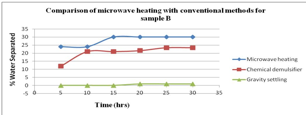
Figure 8b: Comparison of microwave heating with conventional methods.
