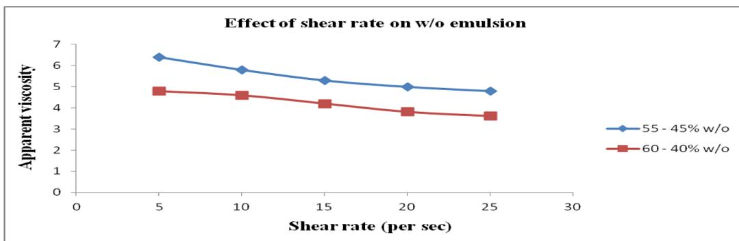
Figure 4: Effect of shear rate on w/o emulsion
