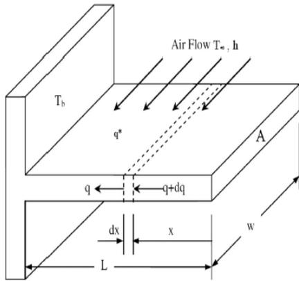
Fig. 1. Schematic of the longitudinal straight fin geometry with the internal heat generation [26]
