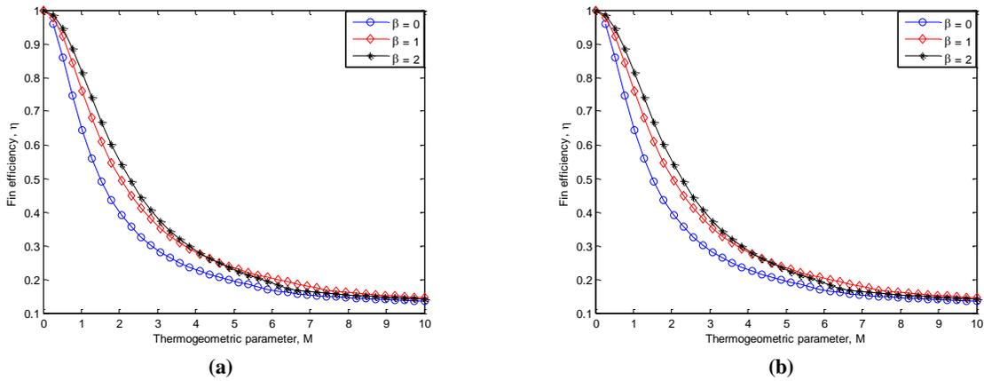
Fig. 4. Effects of thermal conductivity parameter on the efficiency of the fin when (a)  $n=0, Q=0, \gamma=0.2$  (b)  $n=0, Q=0, \gamma=0.8$
