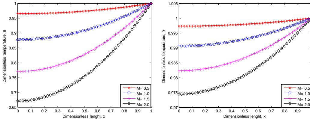
Fig. 2. Effects of thermo-geometric parameter on the temperature distribution in the fin when (a)  $Q=0.4, \gamma=0.2, \beta=0.8$  (b)  $Q=0.8, \gamma=0.2, \beta=0.8$
