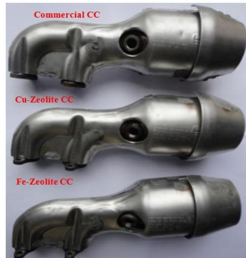
Fig 5 Catalytic converters
