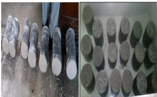
Figure 3. Capping and Curing of cylinders
