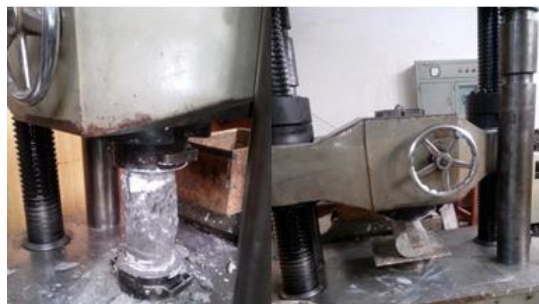
Figure 4. Testing of Specimen in Compression and in tension
