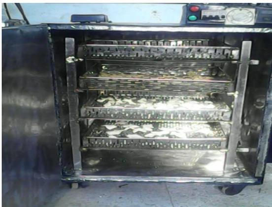
Fig: 2.3: arrangement of the loaded trays on the dryer.
