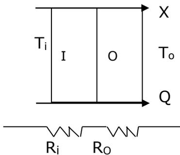
**Fig 4. Heat transfer across a composite slab**
