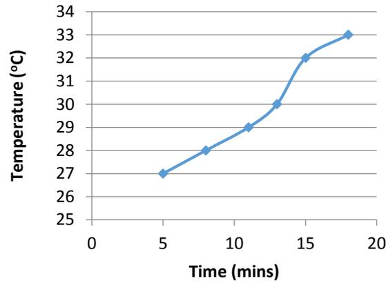
Fig. 5. Temperature rise across the refractory wall
