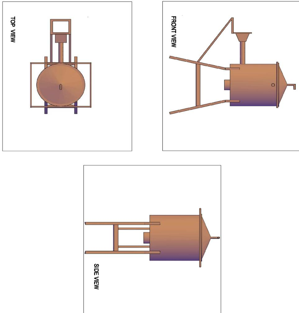
Figure 2 Orthographic Views of the Furnace
