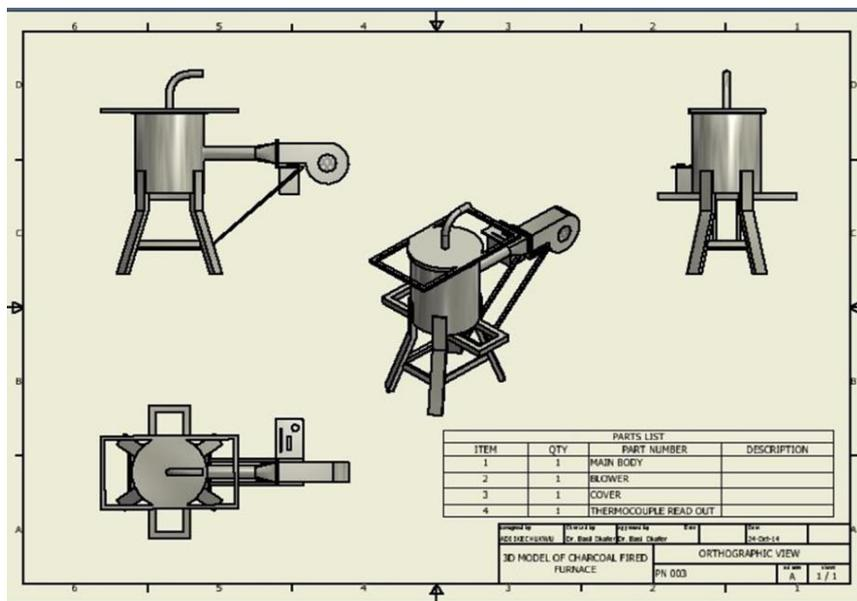
**Figure 1 Assembly views of the furnace**
