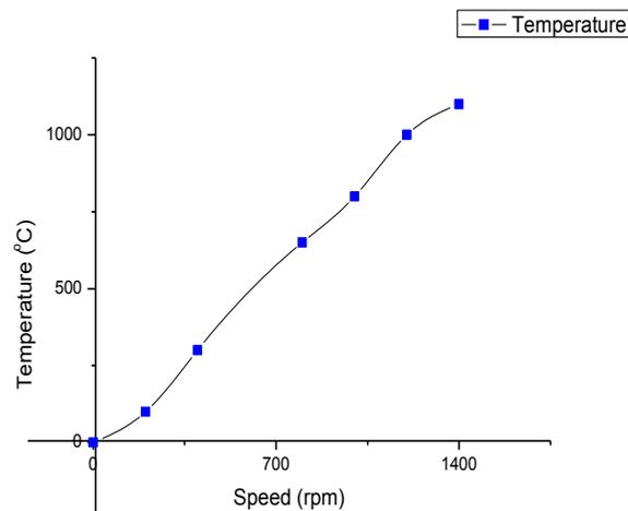
Figure 6.0 Response of temperature with increasing speed of the air blower
