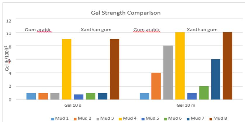
Figure 5 shows gel strength for 10 seconds and 10 minutes measurement for 8 samples
