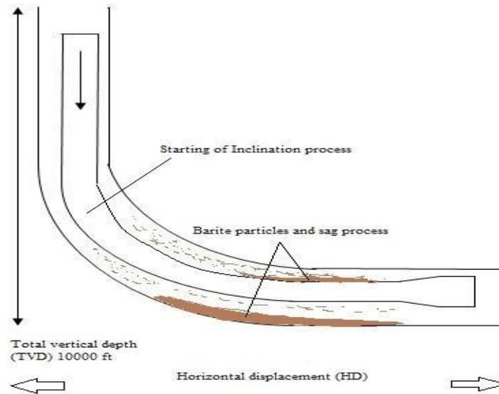
Figure 1 shows the accumulation of barite in directional drilling
