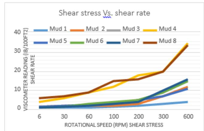
Figure 3 Rheology profiles of fluids measured on the Fann viscometer
