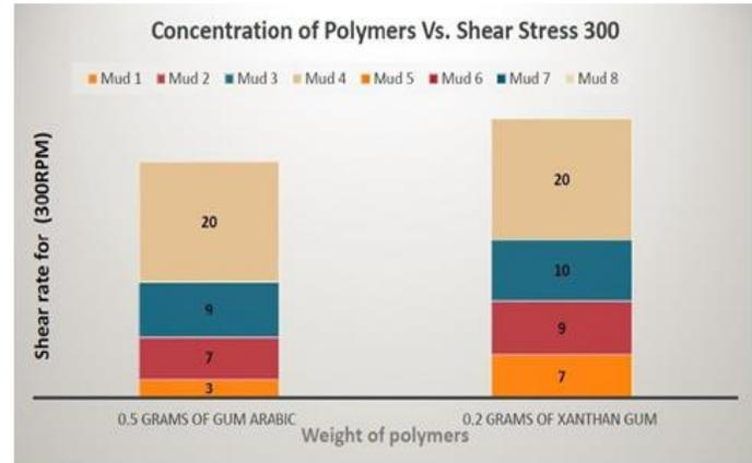
Figure 7 relation between polymer concentrations and shear rate for 300 RPM shear stress
