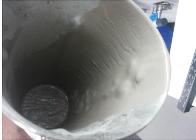
Figure 2 shows barite sag process during the measuring density in the Lab
