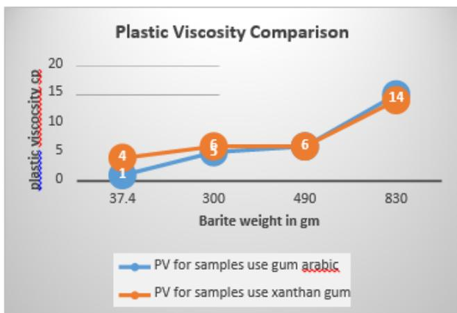
Figure 6 relation between barite weights and plastic viscosity for two type of polymers
