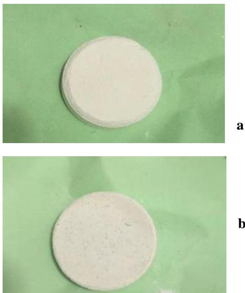
**Fig (3) Samples a) without Cu, b) with 1% Cu**
