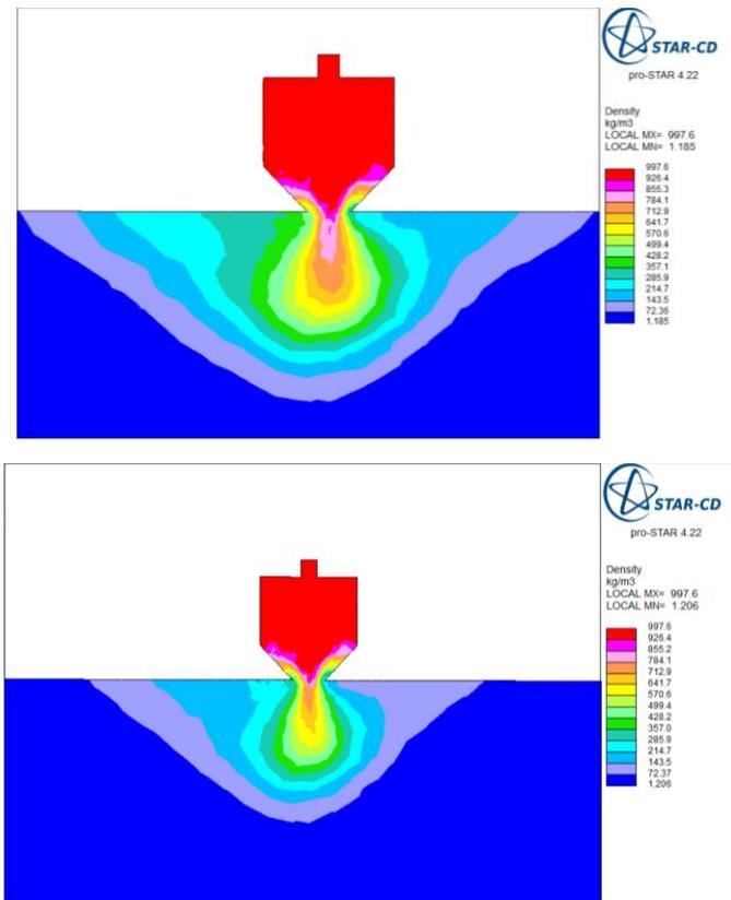
**Fig. 5 Comparison of contour plot of density for SIMPLE and PISO algorithms**
