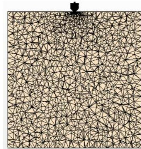
Fig.2 Mesh on vertical plane through the atomizer model
