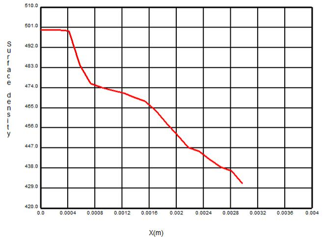
a. Predicted interfacial surface area density at y=5.9 mm
