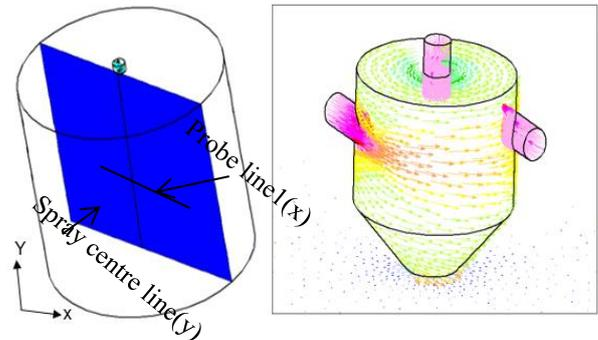
Fig. 3 Vertical section plane and 3D plot of velocity magnitude.
