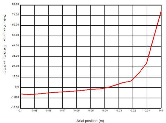
Fig. 8 Droplet velocity on the symmetry axis
