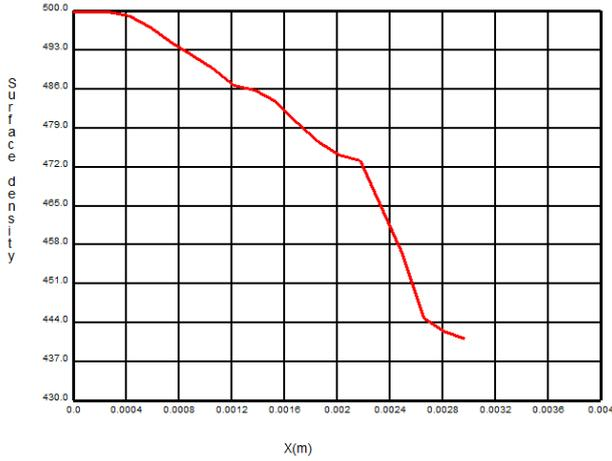
c. Predicted interfacial surface area density at y=5.2 mm
