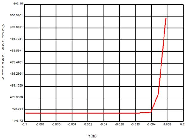
Fig.12. Predicted interfacial surface area density on the spray centre line
