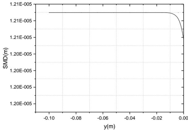
**Fig.14 Spray Sauter mean diameter (SMD) predicted on the symmetry axis**
