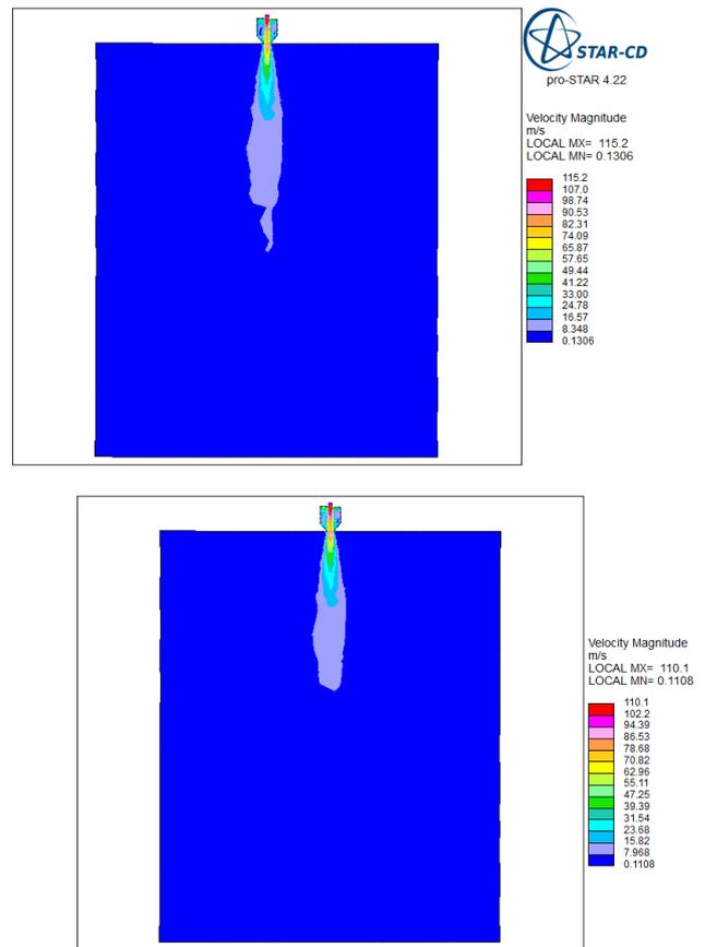
Fig. 6 Comparison of velocity magnitude contour plot on the section plane for SIMPLE and PISO algorithm
