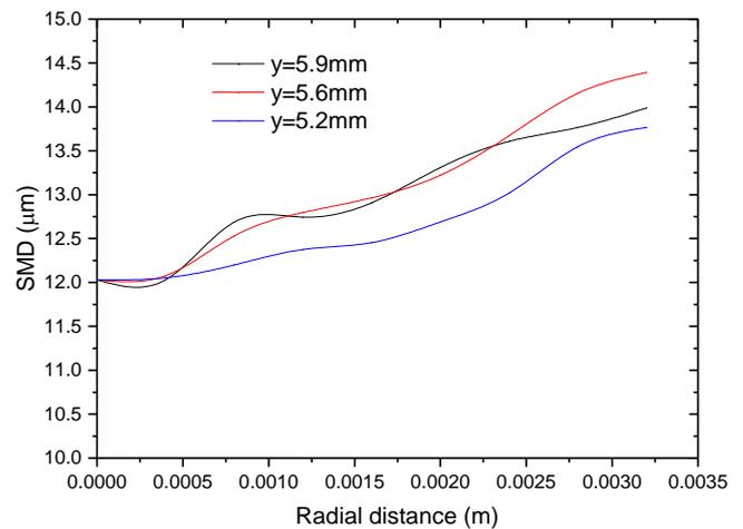
Fig.13 Sauter mean diameter (SMD) at axial positions y=5.9, 5.6 and 5.2 mm
