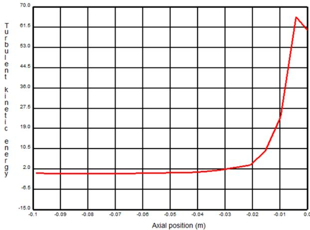
Fig. 9. Turbulent kinetic energy on the symmetry axis
