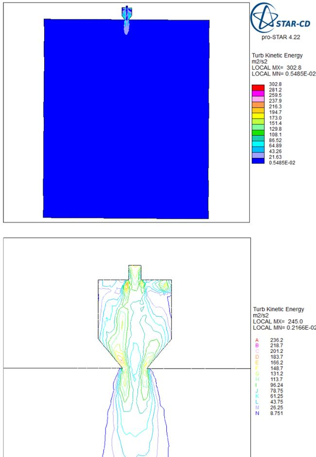
Fig.7 Comparison of turbulent kinetic energy contour plots for SIMPLE and PISO algorithm
